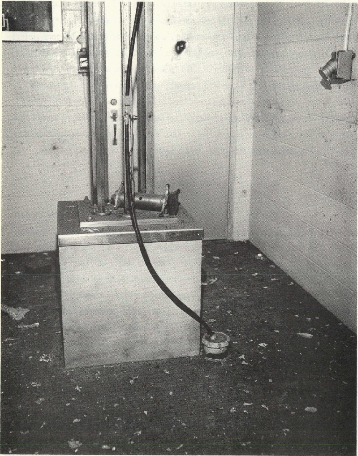
Figure 1. LOX Impact Test Cell after LOX/Asphalt Reaction.
